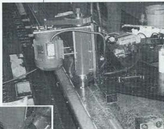
Ingersoll finishing face mill in a 50 taper spindle mounted to a temporary carriage milling a bed way.
