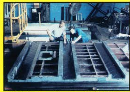
Saddle for Gray floor type HBM finished with oil grooves molded in, completed in 3 days
