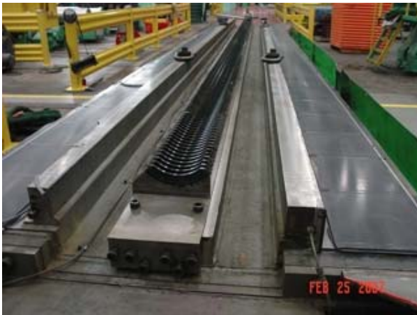
IMAGE 7 The as molded surface before trimming. Also notice that the hydrostatic worm rack segments have been replicated from a master using a moldable bearing material from the OEM
