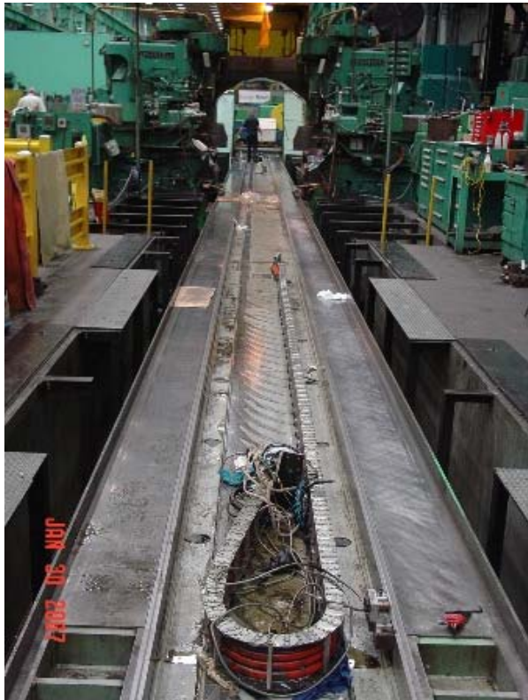
IMAGE 3. 2 ways each 12 inches wide and 140 feet long, fabricated in steel. Notice the horizontal slotting spindles
