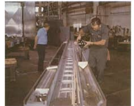
Pouring the Moglice into the bedways
