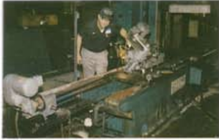
Milling the vee way of a Hill Avme at Pratt & Whitney Machine Tool.
