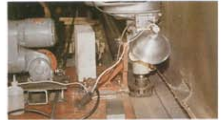
Milling the flat way of a Thompson grinder at Rock of Ages
